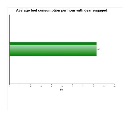
The diagram shows the average fuel consumption based on the operating hours with gear engaged.
