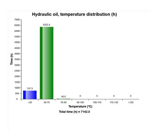
The graph shows the time distribution of the temperature, while engine running.
