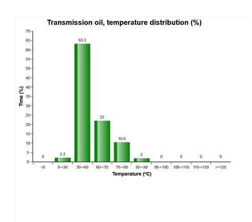
The diagram shows the transmission oil temperature in various temperature ranges. The time is displayed in the following ten temperature ranges:
