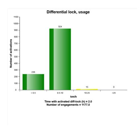
The diagram show, number of times the differential lock has been engaged at each speed interval
