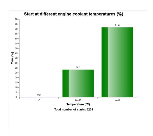
The graph shows the distribution of engine coolant temperature, at the starting moment.
