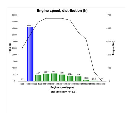
The graph describes the engine speed distribution, compared with the engine torque curve.
